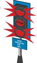
If the indicator is activated, any movement on the line to which the signal applies or any other line, is to be brought to a stand immediately and the signaller contacted.
