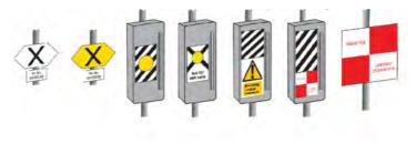
**Note:** A driver of a train at a signal with any of the signs shown above is allowed to use the signal post telephone under specific arrangements.
