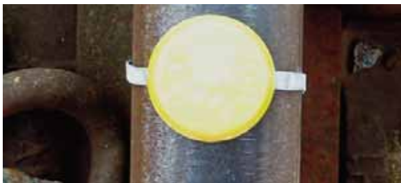
Detonator secured to rail
