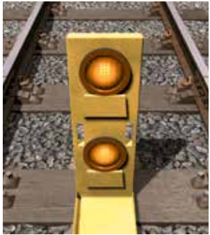
Exit from the worksite
