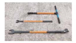
Insulating hand tools are made totally or predominantly from insulating material. The insulating part of these tools is usually coloured orange and will state the BS standard BS8020.
