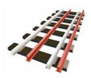
In the London area, lines used by Underground trains are also fitted with a fourth rail located in the four foot. This is also a conductor rail and must be treated as live and dangerous at all times.
