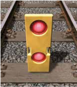
Entrance to the worksite
