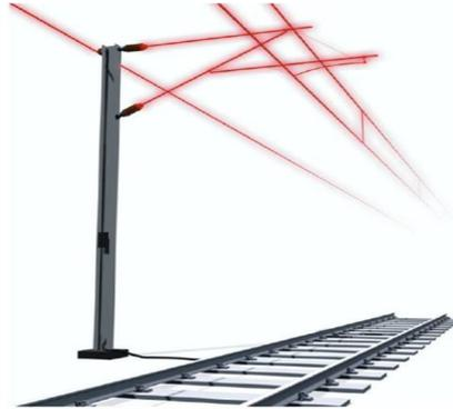
When on a section of line which is adjacent to or passes over NR lines electrified by 25kv (A.C) Overhead Line Equipment (OLE). Always:
