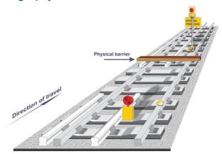
This method of protection can be used in fully un-signalled depots or on un-signalled tracks in other depots. A physical barrier, such as a timber baulk, is placed in the four foot as a warning to train operators that the section of the track concerned is under possession.
