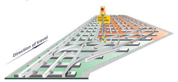
This method of protecting a possession must only be used during Engineering Hours for a minor possession and relies on the Line Clear and Line Safe procedures to provide a protecting 'buffer' traction current section, where traction current is switched off, to prevent unauthorised trains from reaching the traction current section(s), depot or siding under possession.
