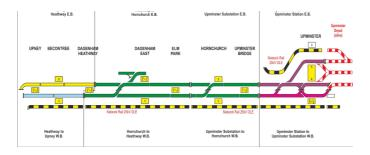
These arrangements utilise Line Clear or Line Safe procedures to provide a method of implementing and removing possessions protection and worksite controls during Engineering Hours.
