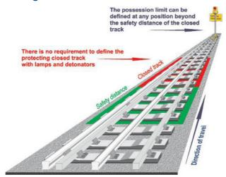
On lines fitted with the Transmission Based Train Control (TBTC) signalling system, signals can be maintained at danger by closing tracks.
