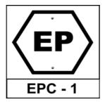
This sign marks the location of the boundary between two TBTC loops. Trains re—entering the TBTC signalling system must ensure that their Vehicle on Board Controllers (VOBC) are reset before passing this sign.
